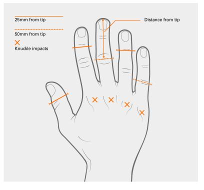
The standard also outlines test requirements, equipment and method **{see Appendix B}**, including preparation of samples and conditioning of the gloves. Within this, it defines specific test sites for the knuckles and fingers and thumbs, and requires that the sites be marked on the outside and back side of the glove **(see Fig. ii)**.
