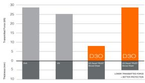
\*When tested at 2.5 J, the 2mm sheet achieved 27.5kN Transmitted Force
