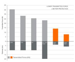
D30<sup>®</sup> AeroMax, Comparative Impact Test (10 J)
