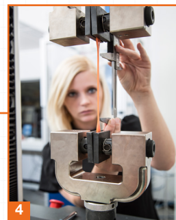
(1) Richard Holman, Material Development Leader for D3O Thermoplastics and Elastomers, trials a new formulation. (2) A piece of motorcycle armor withstands a hammering in the impact rig. (3) Accurate measurements help to show how materials and products are responding to testing. (4) Senior Testing Engineer Aileen McFarlane tests the tear-strength of a new formulation in the tensometer. (5) Moto2 racer Sam Lowes gives his appraisal of the new armor to Principal Product Designer Adam Turvey. Main image: Inside the Material Development Lab.
