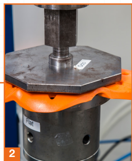
(1) Richard Holman, Material Development Leader for D3O Thermoplastics and Elastomers, trials a new formulation. (2) A piece of motorcycle armor withstands a hammering in the impact rig. (3) Accurate measurements help to show how materials and products are responding to testing. (4) Senior Testing Engineer Aileen McFarlane tests the tear-strength of a new formulation in the tensometer. (5) Moto2 racer Sam Lowes gives his appraisal of the new armor to Principal Product Designer Adam Turvey. Main image: Inside the Material Development Lab.
