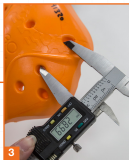
(1) Richard Holman, Material Development Leader for D3O Thermoplastics and Elastomers, trials a new formulation. (2) A piece of motorcycle armor withstands a hammering in the impact rig. (3) Accurate measurements help to show how materials and products are responding to testing. (4) Senior Testing Engineer Aileen McFarlane tests the tear-strength of a new formulation in the tensometer. (5) Moto2 racer Sam Lowes gives his appraisal of the new armor to Principal Product Designer Adam Turvey. Main image: Inside the Material Development Lab.
