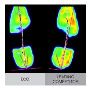
The D3O Insole (left) reduces the pressure felt on the underside of the foot (green = low pressure). The competitor insole (right) fails to match this (red = high pressure). The acceleration control is also maintained much better by the D3O Insole, highlighted by the fact that the black dotted line is more consistent along the pink midline.\*
