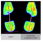
The D3O<sup>®</sup> Insole (left) reduces the pressure felt on the underside of the foot (green = low pressure). The competitor insole (right) fails to match this (red = high pressure). The acceleration control is also maintained much better by the D3O<sup>®</sup> Insole, highlighted by the fact that the black dotted line is more consistent along the pink midline.\*
